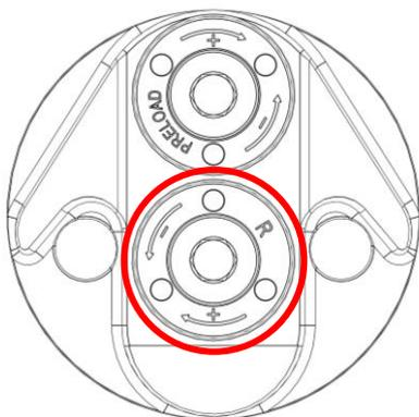
**WARNING:** is necessary to have an allen key ch4 to operate with the adjuster screw. Please don't force beyond the end turn limit of the adjuster.
