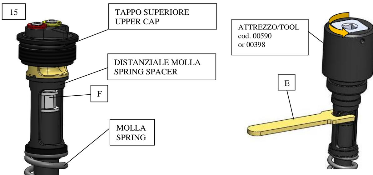
12- Fix the cartridge directly to the fork feet like in the scheme 2. In the low end "G" insert an allen key of 19mm and tight at 28Nm.
