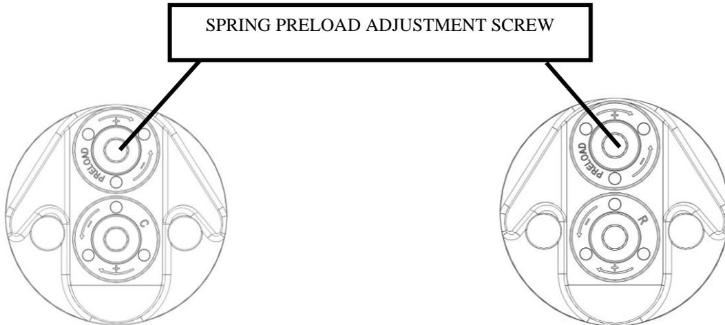
The preload values are very important like the values of the forks strip out. The preload defines the height of the bike from the ground as well as the dynamic set-up on a bend, therefore also the angle values of the fork, the front, etc. which characterize the behaviour of the vehicle. **Generally speaking, the best preload values are defined between 3 and 8 mm.** To optimized the preload values, please read the chapter "Measurements and adjustment of the vehicle Sag"
