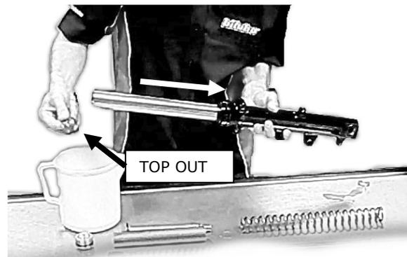
12. Insert the original top out into the lower spacer of the BITUBO cartridge. If you want to use the length reduction KIT, insert also the respective spacers, checking the table in the SHORTENING section (pag. 26).
