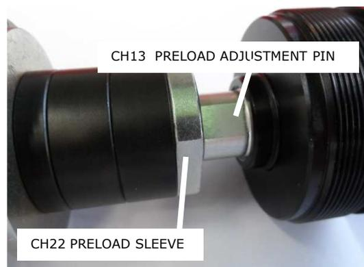
3. Unscrew the preload sleeve the shims are inserted into.
