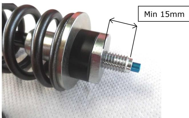
6. Screw in and tighten the cap, carrying out the operations listed in point 2.
