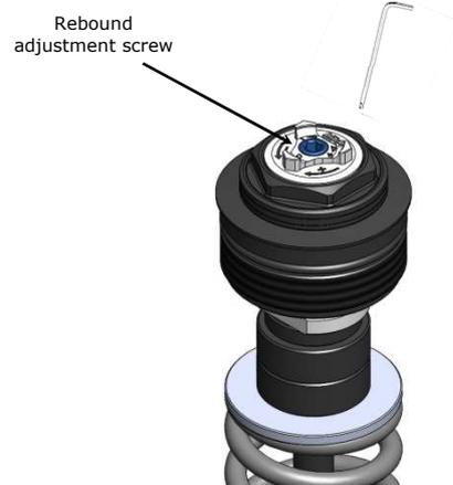
Both adjustments can be performed with a common male hex key with a 4mm spherical head.
