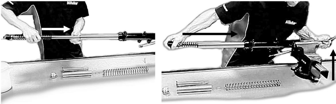
14. Position the cartridge vertically. Pour Bitubo oil code 997630, for the quantity refer to the table "1" in the BASE SET-UP section (pag.1). Perform some compressions and extensions of the fork tube to allow the oil to load correctly. The level is from the edge of the tube, with the tube lowered, the pumping rod lowered and without spring. Check the level references on setting page
