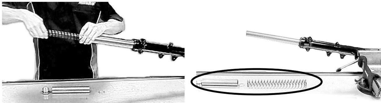
8. Overturn the fork leg and empty the oil from the lower tube.
