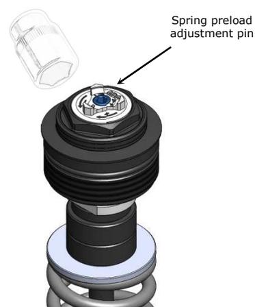
The adjustment of the spring preload can be made with a common 17mm hexagonal bushing.
