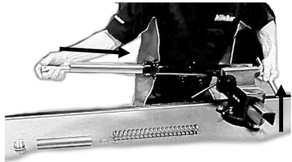
11. Holding the stem at the bottom of the lower tube, take the original piston out with the original top out.
