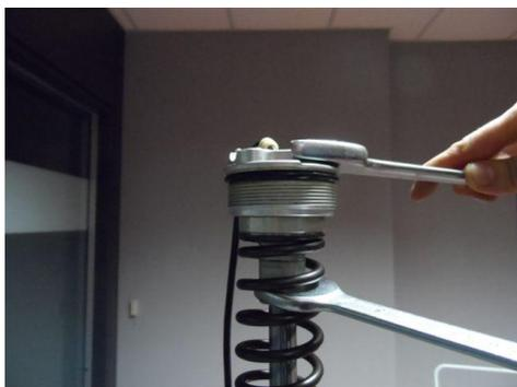
2. Unscrew the ring of the cap from the rod using CH32mm and CH19mm tools.
