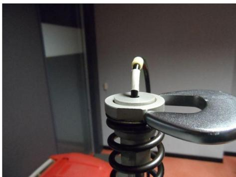
3. Unscrew the spring retainer ring using CH38mm tool.
