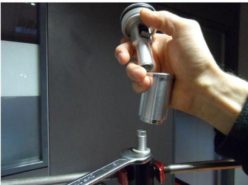
4. Remove the cap and spacer components.
