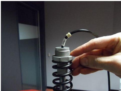
13. Screw the CH38mm ring up to the bottom.
