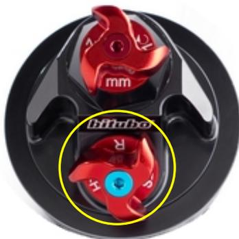
**WARNING:** no specific tools are necessary to operate with the adjuster knob. Please don't force beyond the end turn limit of the adjuster. For rule and coherency with the XXF monoshock, the leg with the hydraulic rebound will be install in the right side of the bike (recognize by the blue screw in the middle of the adjustment knob)
