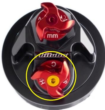
**WARNING:** no specific tools are necessary to operate with the adjuster knob. Please don't force beyond the end turn limit of the adjuster. For rule and coherency with the XXF monoshock, the leg with the hydraulic compression will be install in the left side of the bike (recognize by the yellow screw in the middle of the adjustment knob)
