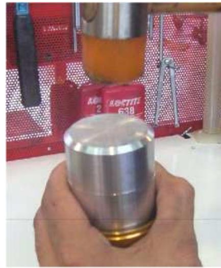
8. Replace the BITUBO support ring in its housing.
