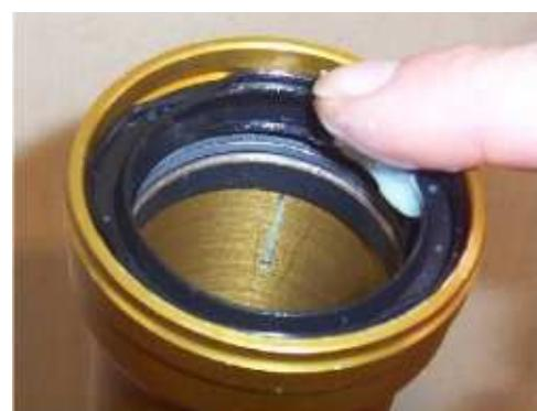
11. Slightly force the seeger in the housing since it will slightly pre-load the oil seal. Make sure that all seeger sides are inserted in the housing.
