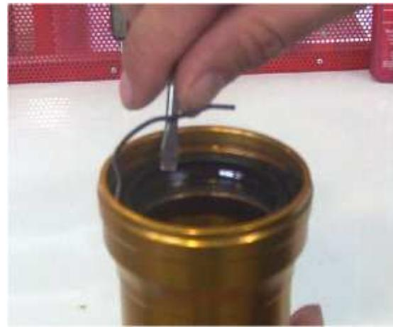
3. Dismantle the oil seal using an appropriate lever.
