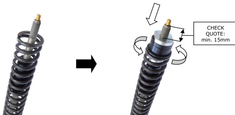
10. Manually screw the top cap in until it rests on the preload sleeve. Tighten the lot to a torque of 9Nm making the opposite operations than the once described in the point **4**.
