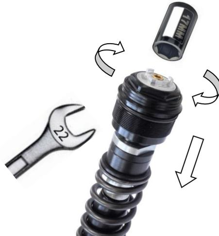
11. Lift the bike forecarriage, making the fork leg stem go up towards the top cap.
