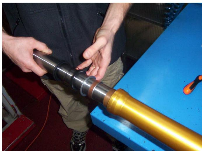
4. To remove the oil seal and dust scraper, the ring on the piston rod must be protected so as not to damage the oil seal when moved: use for example a teflon tape band
