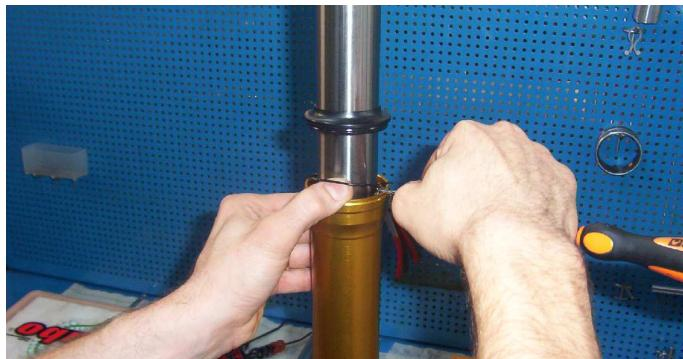
3. Securely lock the foot in a clamp, heat the sleeve in the oil seal area to about 50/60°. Separate the rod from the sleeve moving it in some rapid over-extended movements. Take note of the correctly mounting sequence in the rod of the several components.
