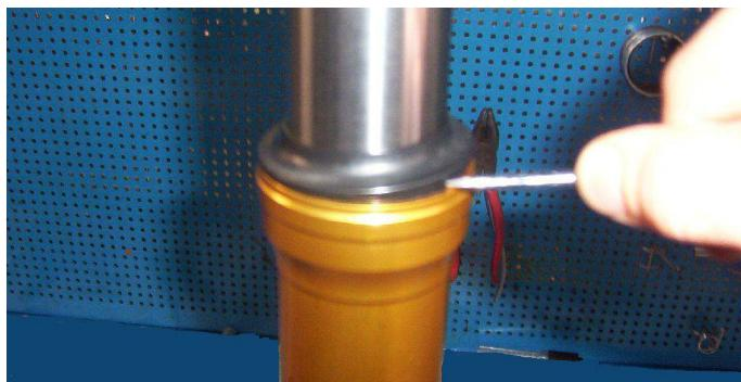
2. Remove the seeger ring making sure not to scratch the sleeve and piston rod.
