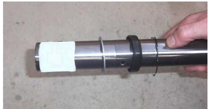
5. Accurately clean the interior of the sleeve and especially the bushing housing with specific detergent. Accurately clean all components.
